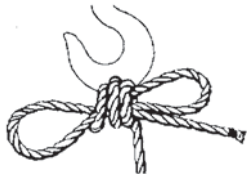
Single snorter shortener partly made. Two bights ready to be placed on hook.
