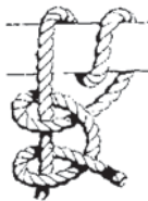
Round turn and two half hitches – widely used for securing running ends of tackles. The more turns made before hitches are made the more control is possible.
