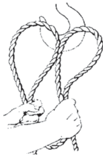
Double shortener for sling on hook.
