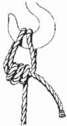
Single snorter shortener with both bights fitted on hook.
